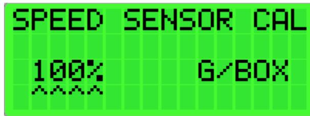
To calibrate the speedometer, press the ADJUST button to change the calibration value by one unit (from a range of 25-250%). Use the following equations to work out what the calibration value should be
